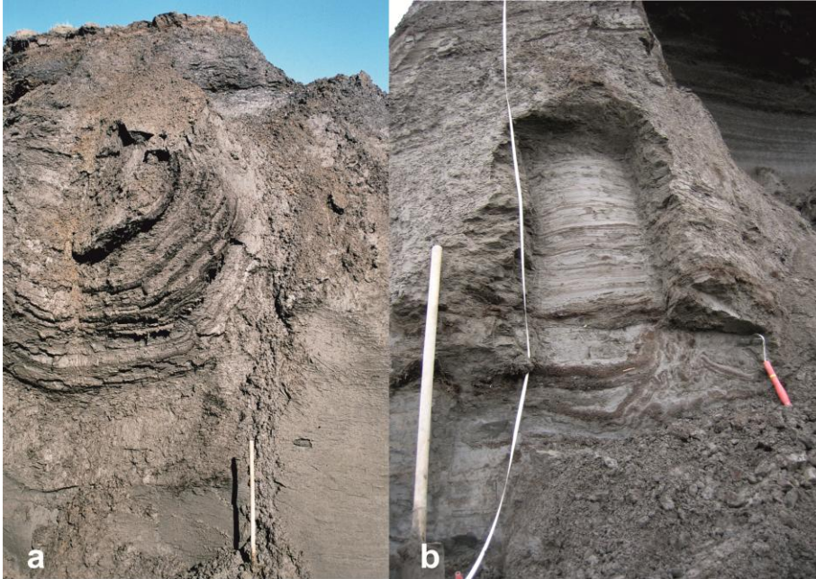
Figure 3. LIG (Krest-Yuryakh) deposits exposed at the southern coast of Bol'shoy Lyakhovsky Island (Figure 2a): (a) ice-wedge pseudomorph (profile L7-11) with well-bedded lacustrine deposits and (b) laminated lacustrine deposits (profile L7-14 A-C) with alternate bedding of peaty and silty sand layers, and a slumping structure (next to the hoe).
