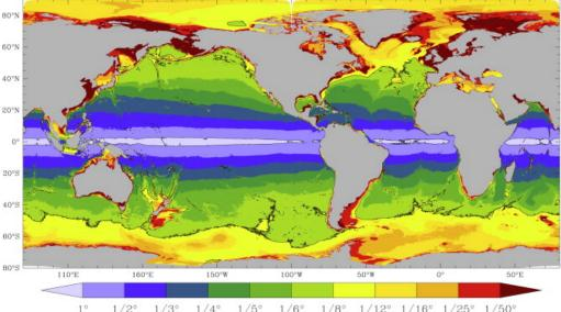
$1^\circ~1/2^\circ~1/3^\circ~1/4^\circ~1/5^\circ~1/6^\circ~1/8^\circ~1/12^\circ~1/16^\circ~1/25^\circ~1/50^\circ$  Mercator Grid Resolution Required to Resolve Baroclinic Deformation Radius with 2  $\Delta x$
