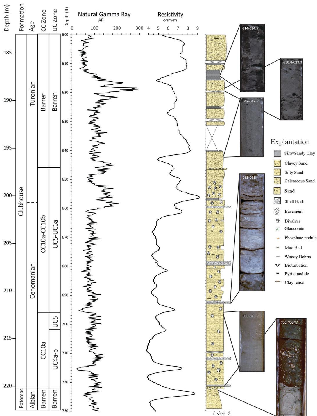
**Figure 2.** Stratigraphic column for Hope Plantation Core with CC and UC calcareous nannoplankton biozones, natural gamma ray and resistivity logs, and representative core images. C = clay; Slt = silt; SS = sand; G = gravel.
