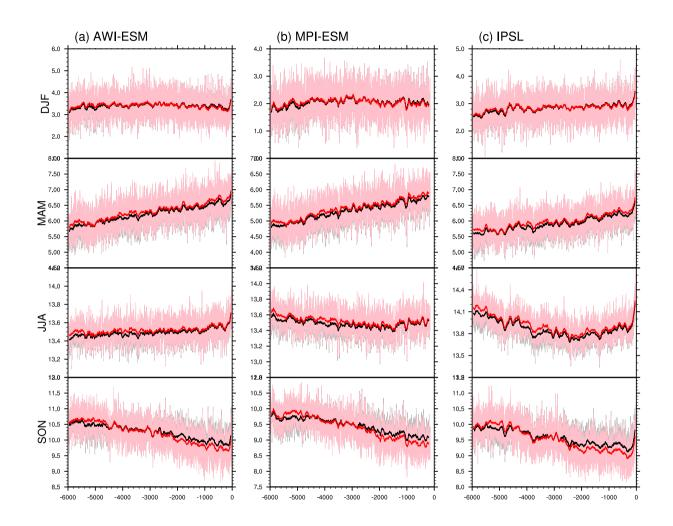
**Figure 13.** Time series of surface air temperature in classical and angular means averaged over Northern Hemisphere oceans, weighted by month length, for (a) AWI-ESM, (b) MPI-ESM, and (c) IPSL-CM. Grey and pink lines stand for the original classical and angular means respectively. Smoothed curves with a running window of 100 model years are shown in black (for classical means) and red (for angular means). Units:  $^{\circ}$ C.
