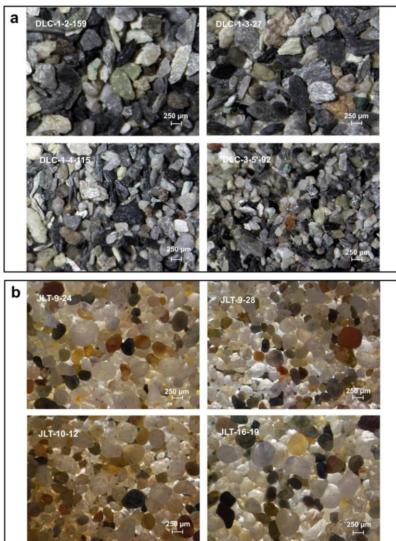
Figure 2. The photomicrograph comparison of 125-500  $\mu\text{m}$  size-fractions in Lake Dalongchi and the typical eolian sand in Jilantai Salt Lake. (a) The 125-500  $\mu\text{m}$  size-fractions from randomly selected samples of DLC1819 core. (b) The typical eolian sand from randomly selected samples of JLT-2010 core (Zhang et al., 2021b).
