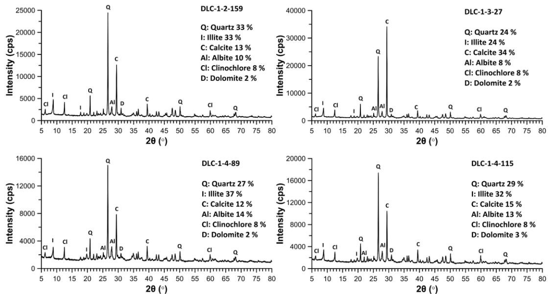
Figure 3. The XRD diffractograms and mineral compositions of 4 randomly selected samples in DLC1819 core
