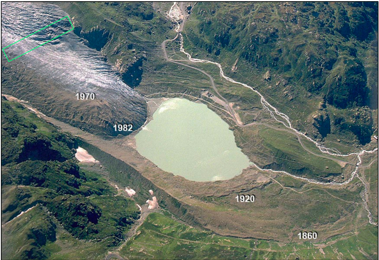
Fig. 4: Aerial photograph of Steingletscher terminus position in 1982 CE with indications of the timing of earlier glacier extents, from www.swisseduc.ch . The location of the Chüebergli sample profile is indicated by the green box . Ice thickness in 1982 CE is estimated at ~50 m to ~20 m above the analyzed samples .
