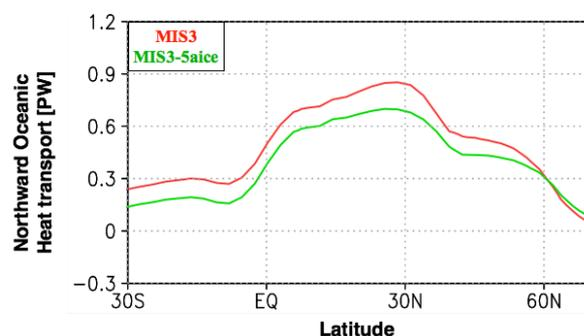
Figure 6: Northward oceanic heat transport over the Atlantic basin simulated from the AOGCM. Red: MIS3 and Green: MIS3-5aice. The climatology of the last 100 years is used to create these figures.
