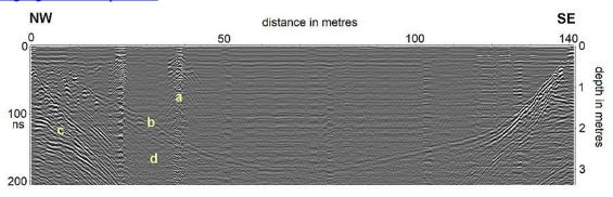
Fig. 3. GPR reflection profile across the Młynek Lake (cf. Fig. 2), a – drilling M-1, b – upper boundary of the so-called hard bottom, c –stratified glaciofluvial sandy-gravel beds beneath the lake sediments, d – attenuation zone of electromagnetic waves connected with occurrence of organic sediment (gyttja) (measurements, processing and interpretation: Fabian Welc).
