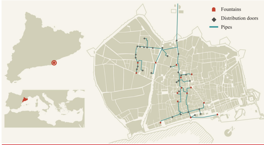
589 590 Figure 9: The urban water supply network of Barcelona as described in the Llibre de les Fonts . Source: 591 Modified from Guàrdia, 2011.
