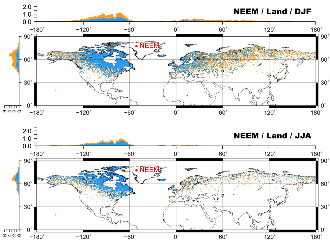
Figure Reply 1. Back trajectory analysis from the NEEM site. Endpoints of 10-day trajectory are plotted for winter (upper panels) and summer (lower panels) by the same manner of Schüpbach et al. (2018). Blue and orange dots denote wet and dry deposition at the NEEM site. Histogram axes indicate contribution to the all endpoints including ocean.
