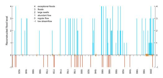
**Figure 8**: Six-point index series of historical flow in the Bermejo River (northern Argentina) between 1600 and 2008 CE based on documentary evidence. These annual-level data were used to create the decadal-scale flood series in Prieto and Rojas (2015). Zero values are indicated by short orange bars.
