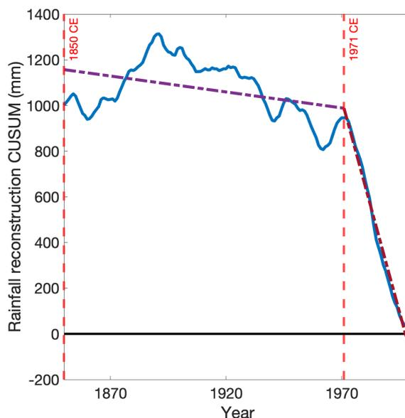
**Figure 5.** CUSUM time series on rainfall reconstruction in period 1850–2000 CE. Yellow dotted lines are each interval’s gradient calculated by using BREAKFIT analysis, with 1971 CE identified as the break-point. The gradient before 1971 CE is -1.40 mm/year. The gradient after 1971 CE is -37.16 mm/year.
