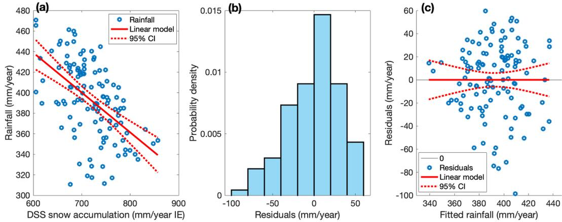
**Figure 2.** (a) The scatter plot for AWAP rainfall in MASK region and DSS snow accumulation (both 6-year window) of period 1900 CE to 2015 CE with their linear model and 95% CI. (b) The histogram for model residuals using probability density function scaling. (c) The scatter plot for model residuals and fitted data with their linear fit and 95% CI.
