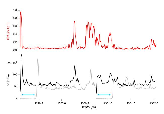
**Figure 5.** Example of the DEP data gap length and relative precision of ECM vs DEP depth assignment. The DEP measurement with a wrong depth in grey and after shifting depth in black. There is a gap of 35 cm (1300.4–1300.75 m) between two DEP measurements. Blue arrows show the early measurements before the starting position of the core. Corresponding ECM data in red.
