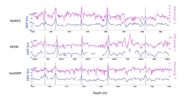
Figure 7. Example of ECM and DEP data matching between the NGRIP2 (top), NEEM (middle) and EGRIP (bottom) cores. The match points are marked by grey bands.
