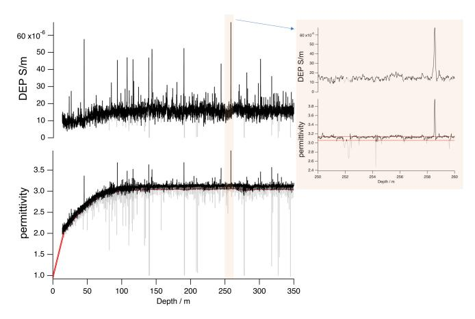
**Figure 4.** Example of DEP data processing (removing core breaks from the raw data). The permittivity measurement is in grey and after processing in black (bottom). The permittivity drops below the red line and shows bad quality of ice-core sections. As seen above (top), corresponding conductivity before processing data (grey) and after processing data (black). The insert shows the details for a short section (250–260 m).
