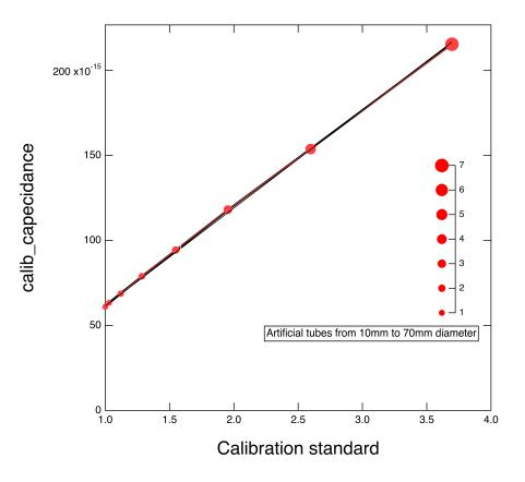
Figure 3. Calibration curve of the measurements with artificial tubes and free-air measurement for DEP device
