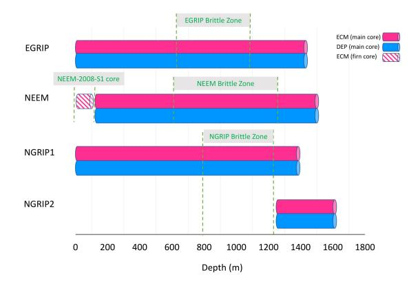
Figure 2. Overview of dielectrical profiling (DEP) and electrical conductivity measurements (ECM) that we used for the synchronization between ice cores over the Holocene and late last glacial periods.
