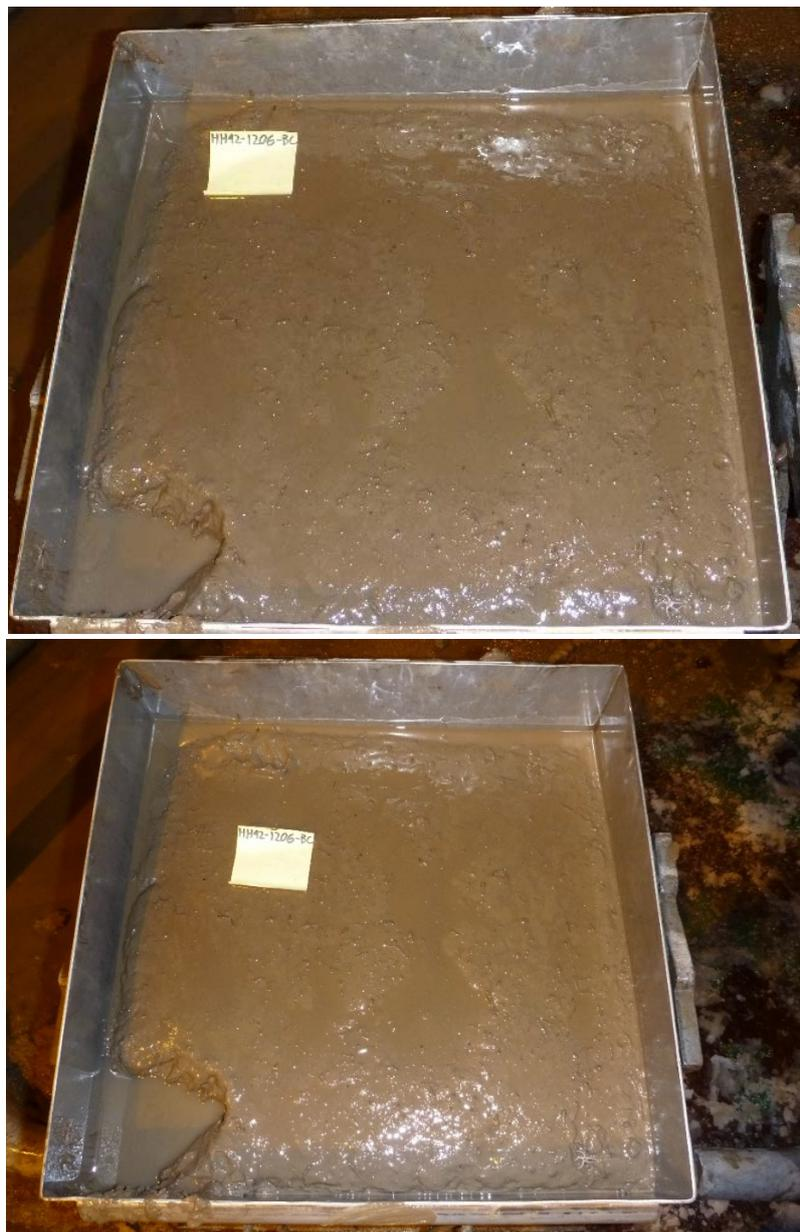
Figure 1. Two photos of the water-sediment interface in box core HH12-1206BC before pushing the tube into the sediment for subsampling. The disturbance in the lower left corner is from removal of the water with a hose.
