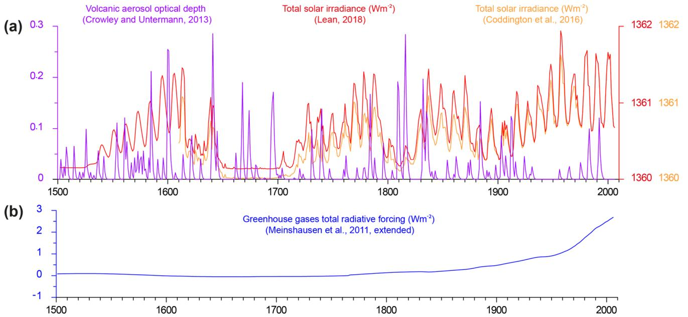
**Figure 2.** Fluctuations in the annual series of external forcing descriptors: (a) volcanic aerosol optical depth and total solar irradiance, (b) greenhouse gases radiative forcing.
