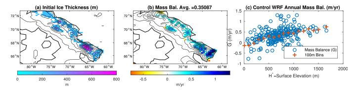
**Figure 1.** Ice thickness and Mass Balance for Ice Sheet Initialization: (a) Ice thickness was adapted from data collected by the NASA Operation IceBridge Mission (Kurtz and Farrell, 2011) with extent set by land use type in WRF. (b) Annual Mass Balance from WRF Control Run.(c) Binned Regression Visualization
