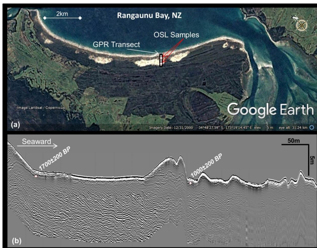
15 Figure 5. (a) Google Earth Image of East Beach, New Zealand, and the prograded barrier that it fronts, with the location of the GPR and OSL collected to study the recent shift in barrier progradation. (b) The stratigraphy imaged in the GPR data shows that while the morphology has been disturbed over this youngest portion of the barrier, the beachfaces prograded normally for a while. OSL was used date the youngest intact relict foredune ridge (1,700 yr BP) and the timing of the drastic shift in evolution observed in both the dune morphology and beach facies stratigraphy (1,000 yr BP). Note GPR is particularly useful to study nearshore dynamics in the stratigraphy at this site, since its location in the high-energy breaker zone makes this region difficult to access and monitor. Figure modified from Dougherty (2011).
