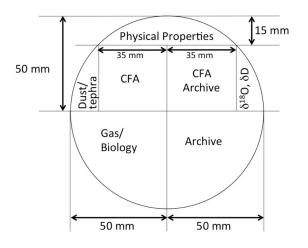
11 **Figure 2:** The RICE main core cutting plan included 2 CFA sticks of size 35x35mm.
