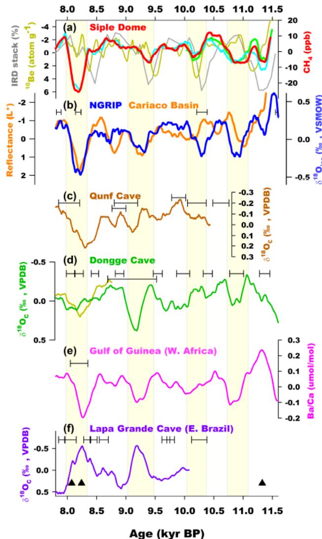
Figure R2. Millennial scale climate variability. All proxies present here were smoothed by 250-year running average and detrended by high-pass filter with 1/1800-year window. (a) Siple Dome CH<sub>4</sub> (red, this study), Greenland <sup>10</sup>Be (dark yellow, Finkel and Nishizumii, 1997), North
