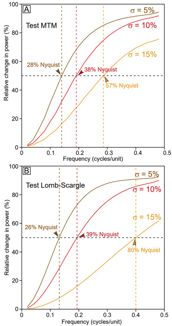
**Figure 4.** Relative change in power in the (a)  $2\pi$ -MTM spectra, and (b) Lomb-Scargle spectra after applying the gamma-law simulations of distortion of the time series. The arrows indicate at which frequency (relatively to the Nyquist frequency) the change in power reaches 50%.
