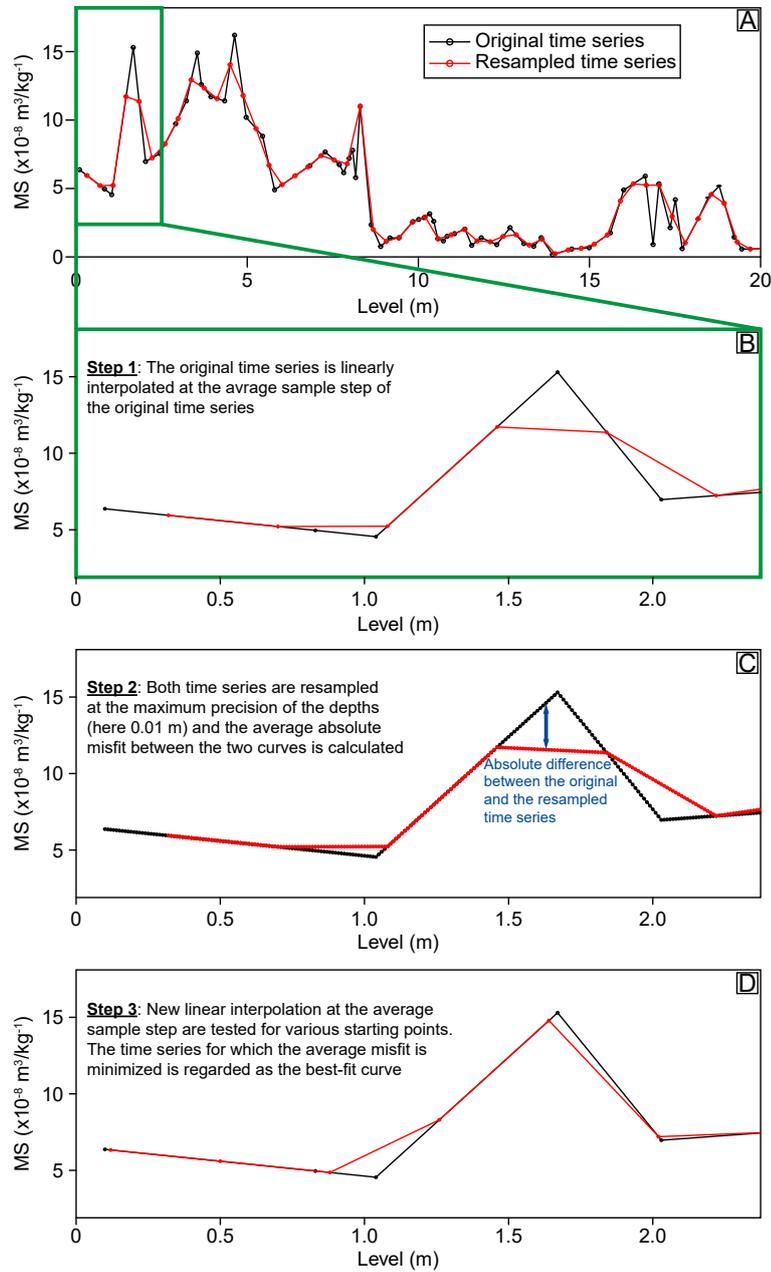
**Figure A.1.** Scheme of the procedure of the optimized linear interpolation of time series.
