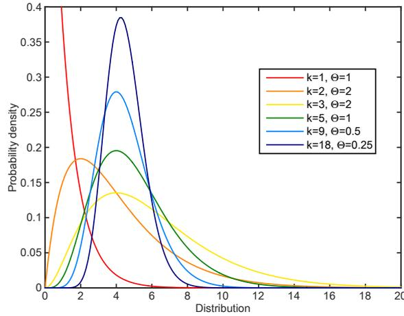
**Figure 2.** Gamma probability density functions (PDF). All Gamma PDF's have a positive support, which is a crucial characteristic to realistically simulate sample steps. The gamma density probability functions were generated with the Matlab *gampdf* function.
