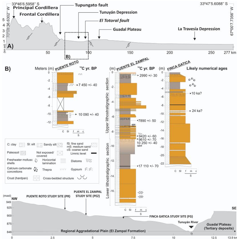
**Fig. 3.** (A) Sketch showing the main morphostructural units of the Frontal cordillera piedmont at the study area (vertical scale is exaggerated). Tunuyán Depression study area is boxed. (B) Schematic topographic profile (adapted from Google Earth software) along the Regional Aggradational Plain in the vicinities of the arroyos Anchayuyo and La Estacada riverbanks. Lithostratigraphic field logs at each study site are shown.
