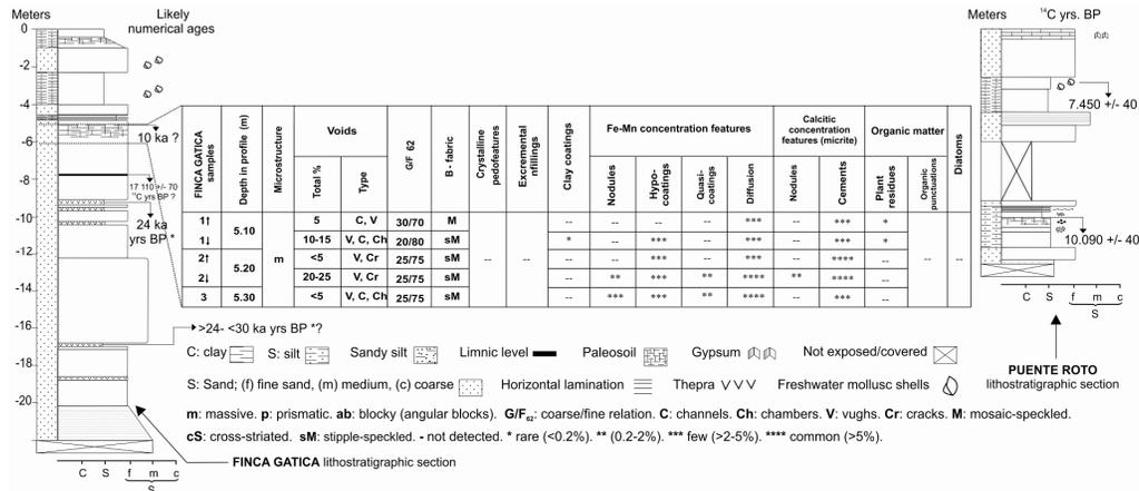
**Fig. 6.** Alluvial sequence field log at Finca Gatica study site (Arroyo La Estacada) and micro-morphology of the ca. 10 ka paleosol. A field log in Puente Roto study site (Arroyo Anchayuyo) is also schematized.
