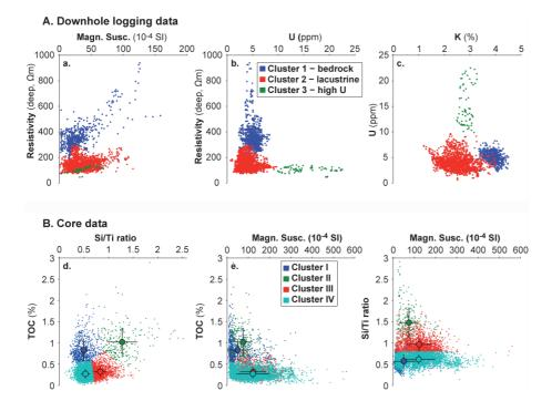
**Fig. 4.** Crossplots of clusters vs. geophysical and geochemical parameters. Upper panel: clusters 1 to 3 derived from k-mean clustering of downhole logging data (electrical resistivity (deep and shallow), magnetic susceptibility, U, Th, and K counts). Lower panel: clusters I to IV derived from k-mean clustering of core data (TOC content, Si/Ti ratio, magnetic susceptibility). In the lower panel, mean and standard deviation of parameters are shown for each cluster.
