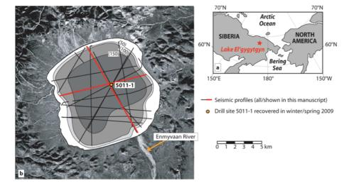
**Fig. 1.** Geographical map of the investigation area. **(a)**: location of Lake El'gygytgyn in NE Russia, **(b)**: aerial photograph of the lake surroundings with lake bathymetry and seismic profiles. The profiles marked in red are shown in Figs. 2 and 3. The orange arrow marks the Enmyvaan River, the only outlet of the lake. Drill site ICDP 5011-1 is shown as an orange circle.
