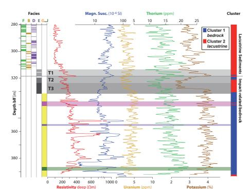
**Fig. 5.** Facies and downhole logging data of the transitional zone between impact-related bedrock and lake sediments. Facies description as in Fig. 3. Clusters derived from k-mean clustering of downhole logging data are shown in blue for Cluster 1 (= bedrock) and red for Cluster 2 (= lacustrine). The impact breccia/suevite succession according to Koeberl et al. (2012) is given as follows: yellow: suevite; lilac: upper volcanic rock layer; violet: lower volcanic rock layer, green: ignimbrite.
