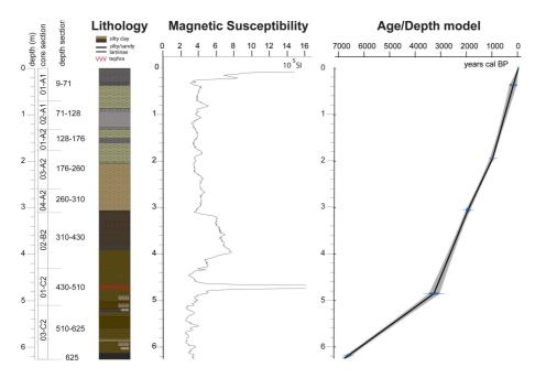
**Fig. 2.** Lago di Pergusa: PG2 core. Lithology, Uncalibrated Volume susceptibility, linear interpolation of AMS calibrated dates. A thin black layer, observed in the section 01-C2, corresponds to the ash event dated in PRG1 at  $3055 \pm 75$  yr BP (Sadori and Narcisi, 2001).
