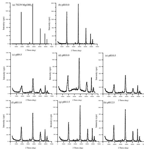
**Fig. 7.** X-Ray diffractogram of brucite deposited from artificial seawater at different pH values. (a) XRD of brucite standard, (b) XRD of brucite from boron-free artificial seawater at pH 10.0, (c-h) XRD of brucite in our experiments. The brucite peak in our samples is clear compared with brucite standard (Fig. 7a).
