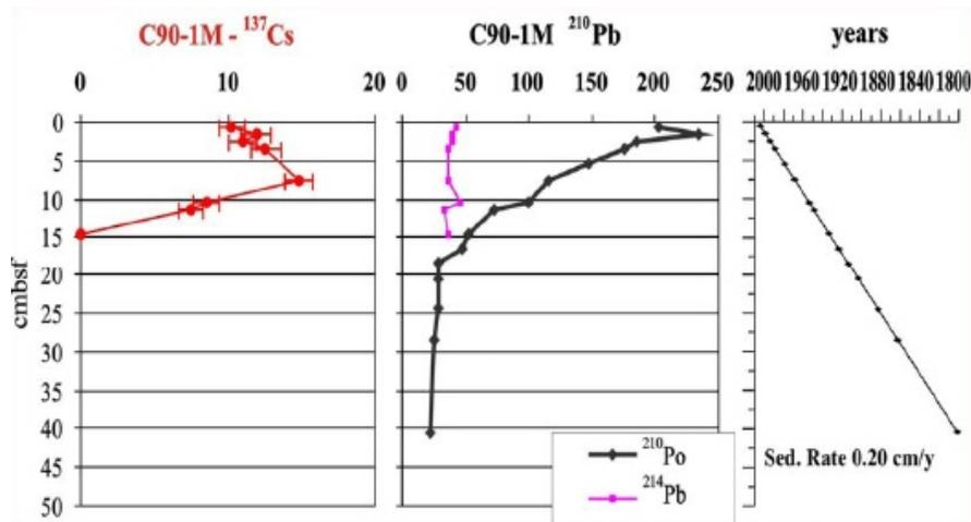
**Fig. 2.** The  $^{210}\text{Pb}$  and  $^{137}\text{Cs}$  activity-depth profiles in core C90-1M and the age-depth profile for the first 40 cmbsf (Vallefuoco, 2008).
