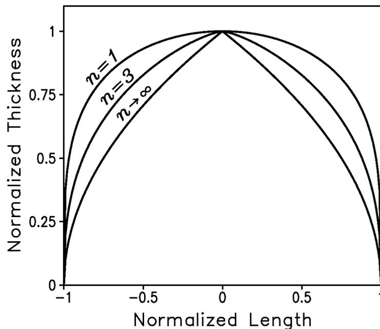
**Fig. 9.** Ice-sheet profiles for illustration of their dependence on the exponent in Glen's law. The  $x$ -axis indicates normalized ice thickness and the  $y$ -axis displays the normalized horizontal expansion on an ice sheet. Typical thickness is some kilometres and typical length some 1000 km.
