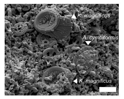
**Figure 4.** SEM picture of the Stevns-1 chalk. Sample 6146 (late Maastrichtian cooling episode, nannofossil subzone UC20b-c<sup>BP</sup>, depth: 73.91 m). Two of the main cool-water nannofossils taxa are shown. Bar is 10  $\mu$ m.
