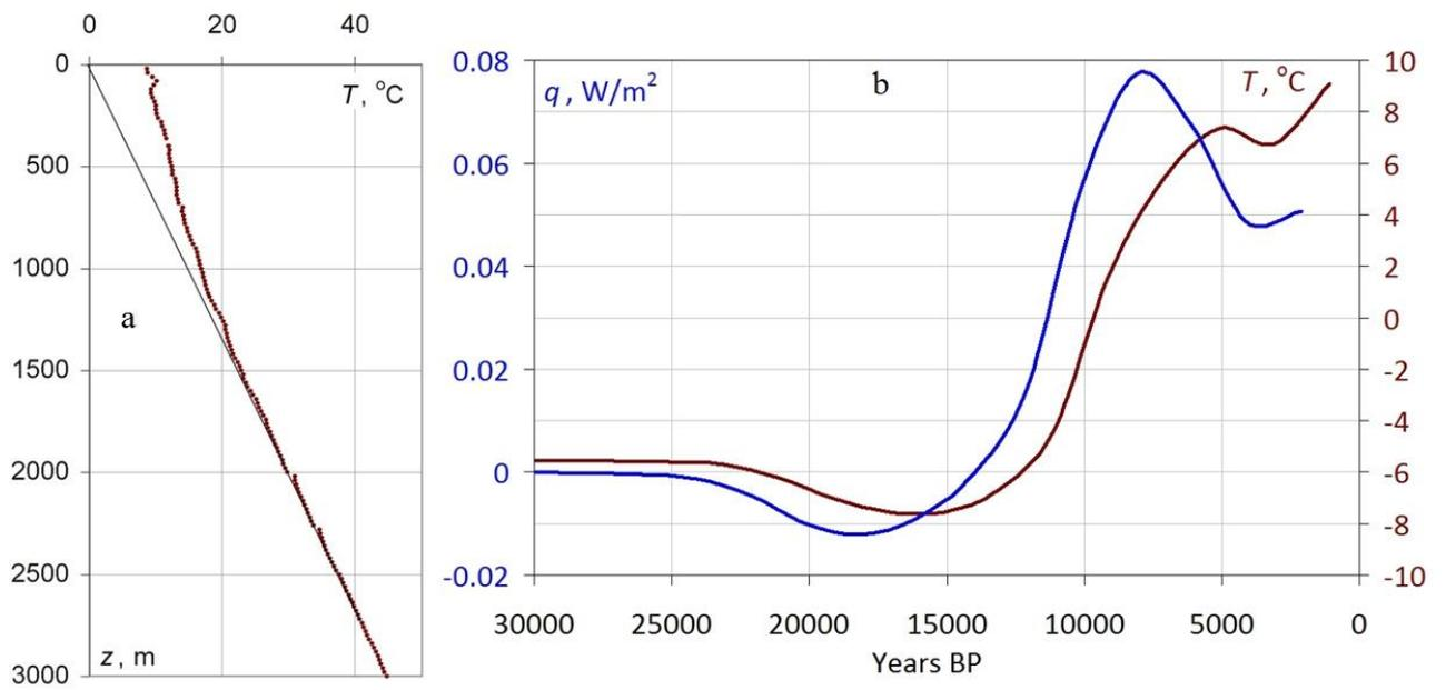
Figure 2. Initial data and surface heat flux a) Temperature-depth profile from the borehole SG-4 (Demezhko and Shchapov, 2001, brown line), b) GST history  $T(t)$  ( $a = 1.0 \cdot 10^{-6} \text{ m}^2/\text{s}$ , Demezhko and Shchapov, 2001, brown line) and calculated according to Eqs. (1-5) SHF history  $q(t)$  ( $E = 2500 \text{ J} \cdot \text{m}^{-2} \cdot \text{K}^{-1} \cdot \text{s}^{-1/2}$ , blue line).
