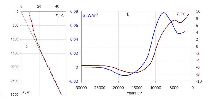
Figure 2. Initial data and surface heat flux a) Temperature-depth profile from the borehole SG-4 (Demezhko and Shchapov, 2001, brown line), b) GST history T(t) ( $a = 1.0 \cdot 10^{-6}$  m<sup>2</sup>/s, Demezhko and Shchapov, 2001, brown line) and calculated according to Eqs. (1-5) SHF history q(t) (E = 2500 J·m<sup>-2</sup>·K<sup>-1</sup>·s<sup>-1/2</sup>, blue line).
