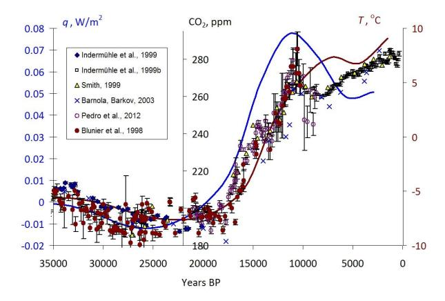
Figure 4. The comparison of GST history T(t) (brown line), SHF history q(t) (blue line) and CO<sub>2</sub> concentration in the Antarctic ice cores (multicolored markers).
