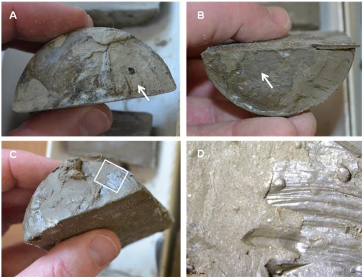
1 2 Figure 6. Concentric grooves in various parts of the Wilson Lake B core, as seen in half - 3 round specimens from the archive half. A: top of a core disc with patches of adhering injected 4 slurry and concentric grooves (highlighted with arrow). B: base of a core disc with patches of 5 adhering injected slurry and concentric grooves (highlighted with arrow). C: top of a core disc 6 with patches of adhering injected slurry and concentric grooves. D: Microscopic detail of 7 highlighted area in C showing a patch of remaining slurry (to the left) unconformably 8 overlying the surface of a core disc which shows concentric grooves. Similar observations 9 were made at other levels in the core.
