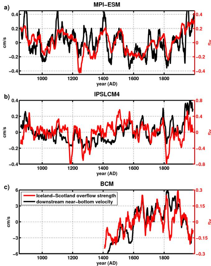
**Figure 2.** Simulated anomalous overflow transport across the ISR (red line; in Sv, 1 Sverdrup =  $10^6 \text{ m}^3 \text{ s}^{-1}$ ) and near-bottom flow speed  $(u^2 + v^2)^{1/2}$  downstream of the ISR (black line; in  $\text{cm s}^{-1}$ ) in MPI-ESM (a), IPSLCM4 (b) and BCM (c). All time series are annual values with a 21-year running mean filter applied.
