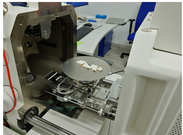
Figure A5. Hitachi SU3900 SEM with an extra-large chamber. The sample holder has a diameter of 28 cm, which is shown here with slab 6 of core KNFa.
