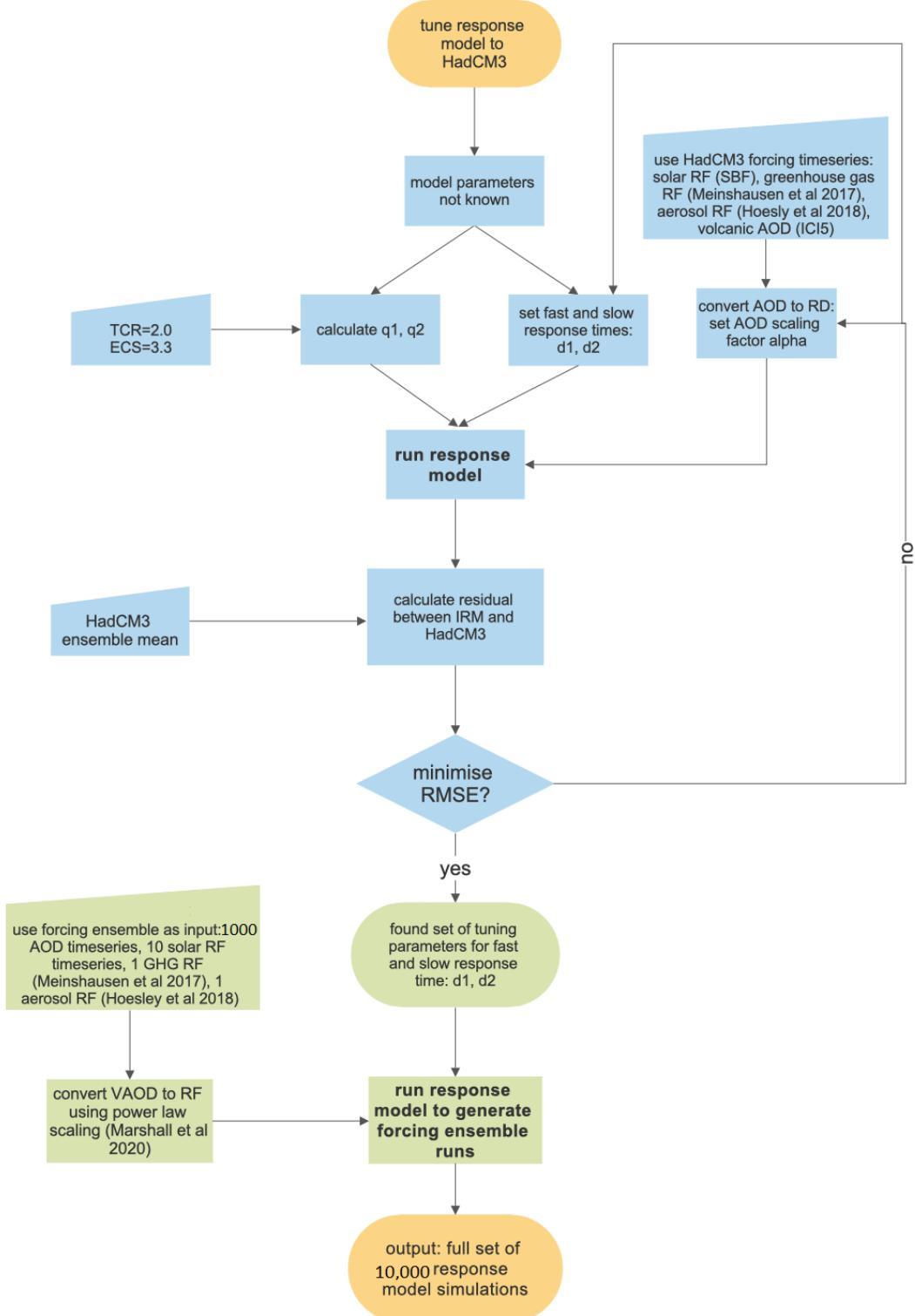
**Figure S7.** Flowchart of the tuning process (blue) followed by the generation of the forcing uncertainty ensemble simulations (green).
