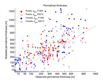
**Figure 6.** Scatter of modeled and observed permafrost thickness estimated from boreholes. Permafrost thickness data for Canada (blue) are from Smith and Burgess (2004) and for Siberia (red) from Melnikov (1998). Filled circles represent modeled permafrost thickness using the Pollack et al. (1993) and open circles using the Davies (2013) geothermal heat flux.
