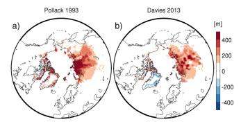
**Figure 16.** Present-day permafrost disequilibrium for the two model runs with different geothermal heat fluxes: (a) Pollack et al. (1993) and (b) Davies (2013). The equilibrium permafrost thickness is computed numerically as outlined in Appendix B, and the actual permafrost thickness is from the transient model simulations of the last eight glacial cycles.
