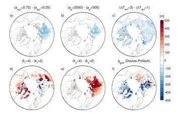
**Figure 7.** Sensitivity of present-day permafrost thickness to surface porosity (a), exponential decay scale of porosity with depth (b), temperature interval for ground freezing (c), rock (d) and dry sediments (e) thermal conductivity and geothermal heat flux (f).
